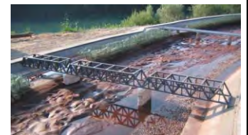
Sediment transport in the physical hydraulic model
